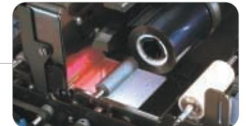
The printhead assembly can be raised for easy ribbon replacement.
